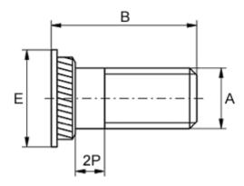
For plate thickness, min = 1.5 Head diameter E = 8 Hole diameter +0.1 = 6.4 Length B = 14 Male thread A = M5x0.8
